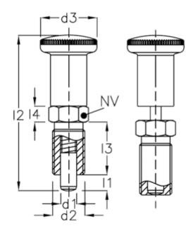
d1 = 5 NV = 12 d2 = M10x1 Spring pressure N bottom = 18.0d3 = 19 Spring pressure N top = 5.0
